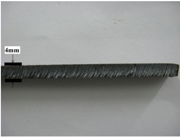
Fig. 2 Cut surface considered good in the 4 mm steel plates
